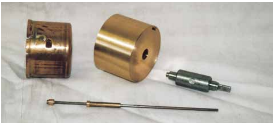
Figure 8 (below). Finished barrel ready for testing. All repairs to clock movement are complete but needing cleaning.
