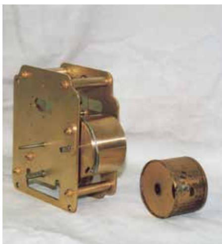
Figure 8 (below). Finished barrel ready for testing. All repairs to clock movement are complete but needing cleaning.
