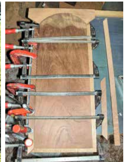
Figure 6. Constructing the trunk door.
