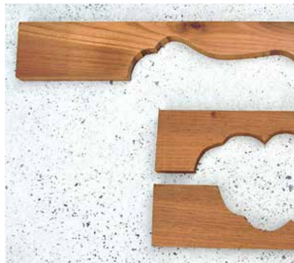
Figure 4. Cut-out for plinth moulding.
